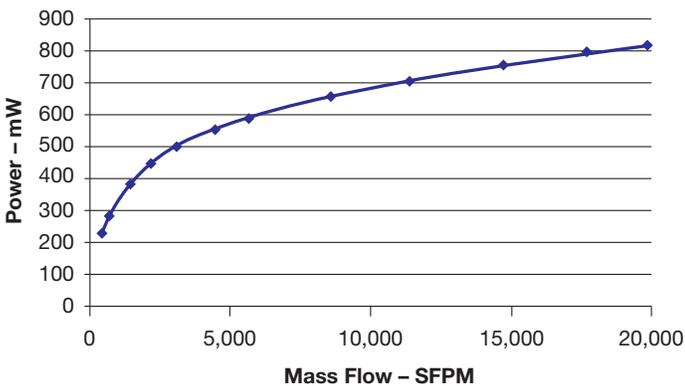
As shown, at low mass flow rates, there is little heat transfer, and thus the amount of power required to maintain the desired temperature difference is low. As the mass flow rate increases, the amount of power required to maintain a constant temperature difference increases.
