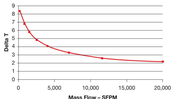
The change in temperature difference with mass flow rate is very large at the low flow rates—this provides the excellent low flow sensitivity.
