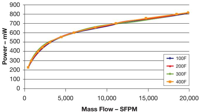
Some thermal mass flow manufacturers compensate temperature only at the electronic circuit. What these manufacturers overlook is that the gas properties that affect convective heat transfer are temperature dependent. Therefore, changing temperature changes heat transfer. MAGNETROL provides real-time temperature compensation that measures the temperature of the gas, and automatically corrects the mass flow measurement based on temperature variations.
