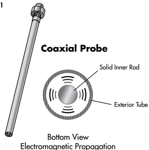
This unimpeded movement of pulses is critical to the concept of overflow-safe probes. With this unimpeded movement and careful design of the upper probe seal assembly comes the fact that there is simply no adverse interaction of signals. With no adverse interaction of signals, the true level signal can always be accurately detected. As shown in **Figure 2**, the level signal is shown unaffected all the way up to the process flange.
