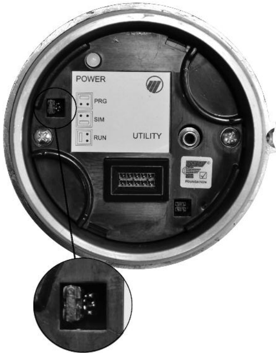
Remove jumper to disable simulation
